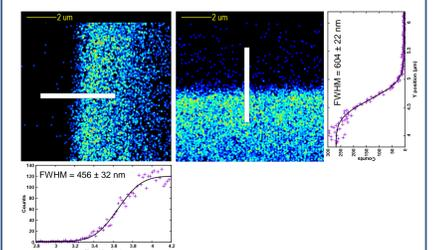
The Cu grid edge definition is not good enough for measuring ~100 nm spot sizes. So, we only use this grid for scan size calibration.
