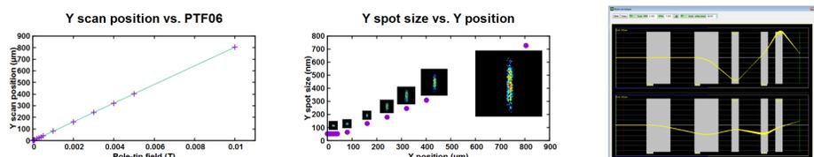
The beam scanning is perfectly linear up to 800 μm offset.
